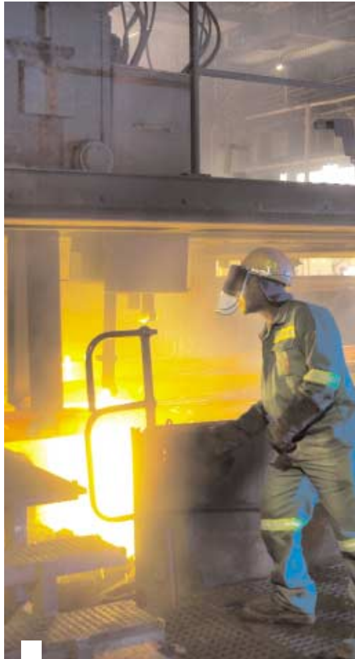
Clean-burning, cost-competitive pipeline gas marketed and supplied by Sasol Gas has important industrial uses. Here, it is being used by Scaw Metals Ltd, near Johannesburg, for hot cutting steel billets.
